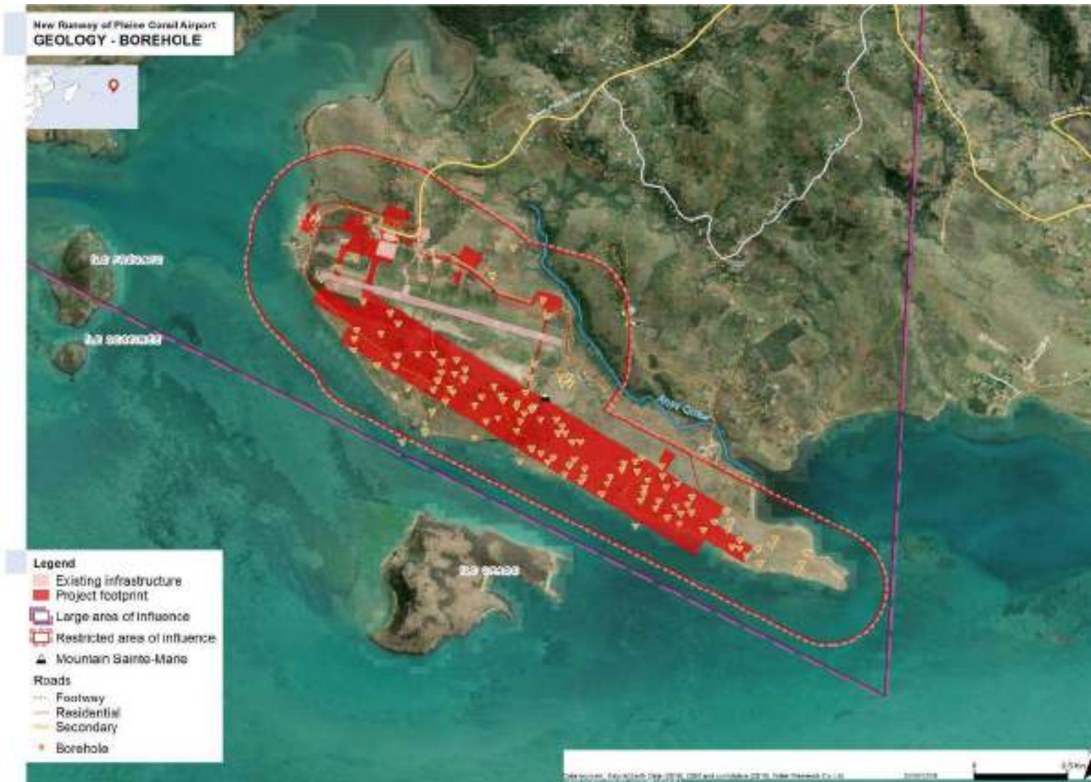
Figure 47: All ground investigations from Phase B (2017) and Phase C (2018) geotechnical campaign of the restricted area of influence at Plaine Corail (Preliminary Design, 2017)
