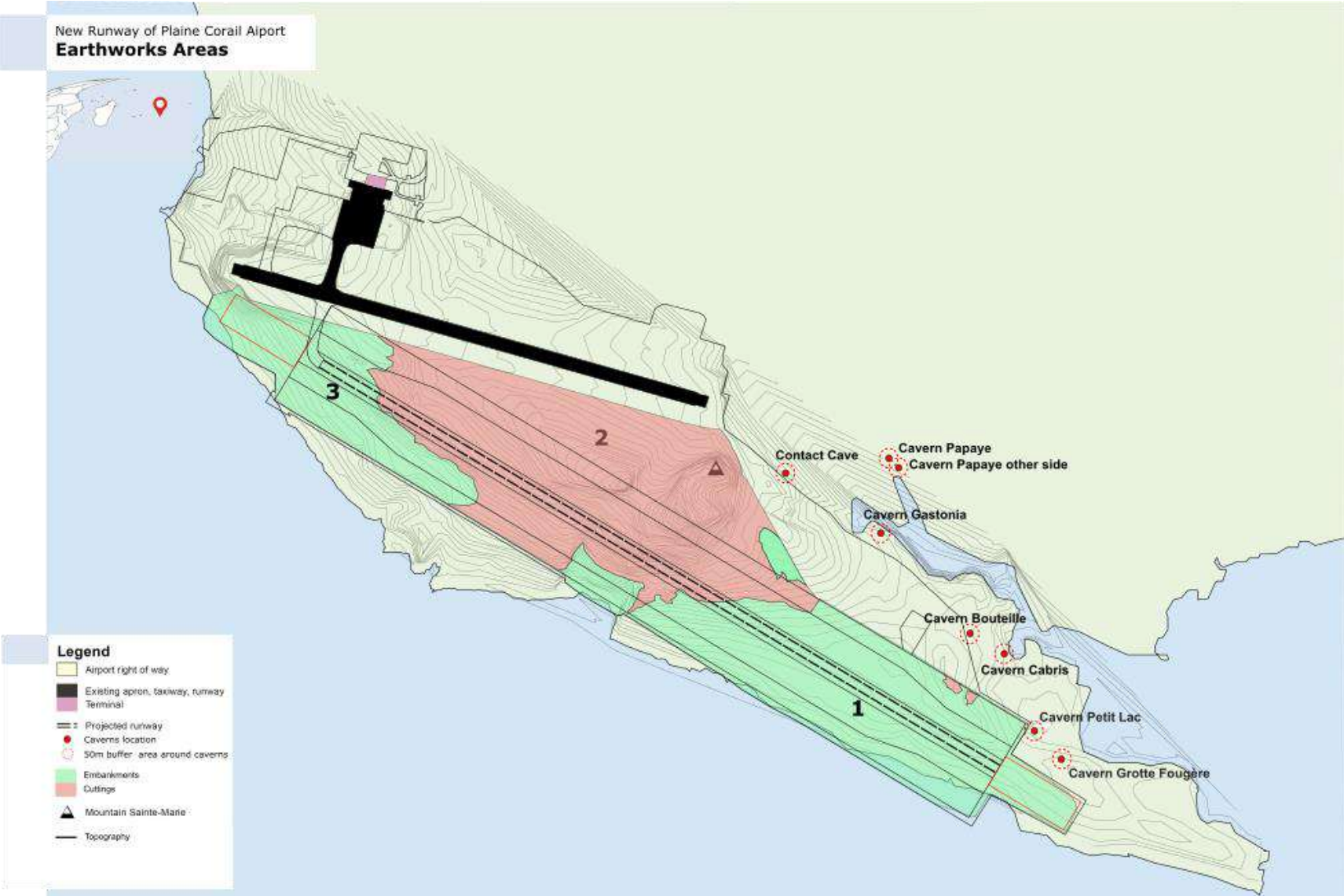
Figure 172: Earthworks areas in the restricted area of influence at Plaine Corail
