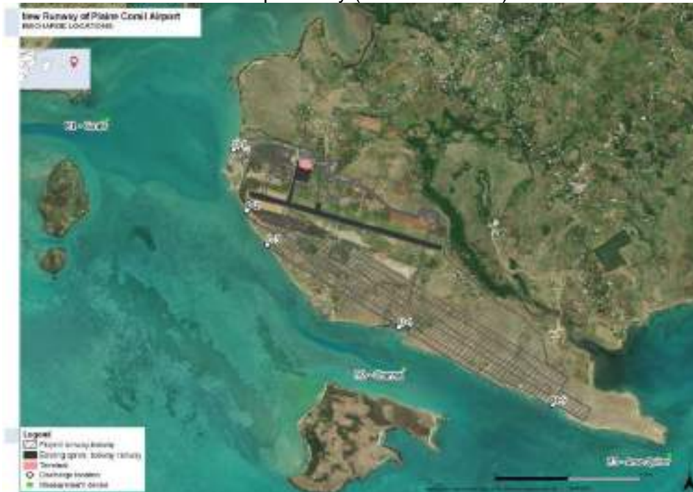
Figure 188 Localization of the potential sediment discharges to the lagoon during works phase and current-meter
